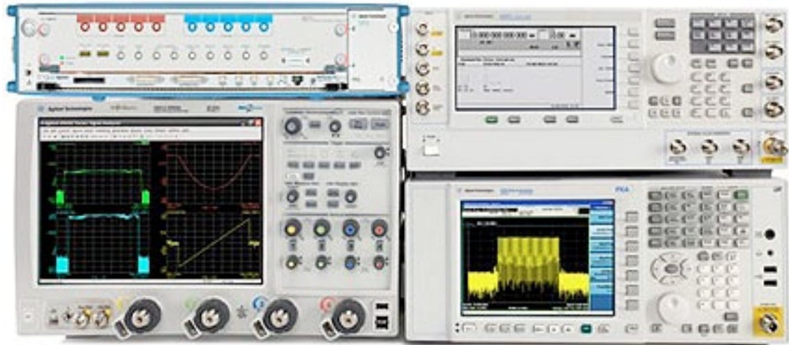
Figure 1. This test setup enables receiver and transmitter testing
