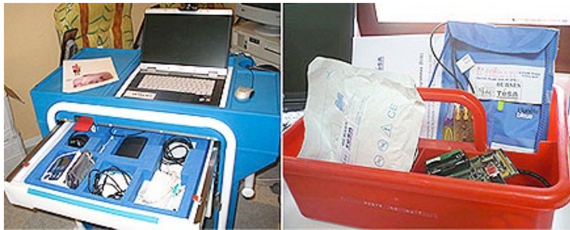
Left: the nurse's trolley, specifically designed for the OURSES project, can be used to send the collected data to each patient's GP. Right: the portable 'TeSA basket' vital signs remote-monitoring system.
