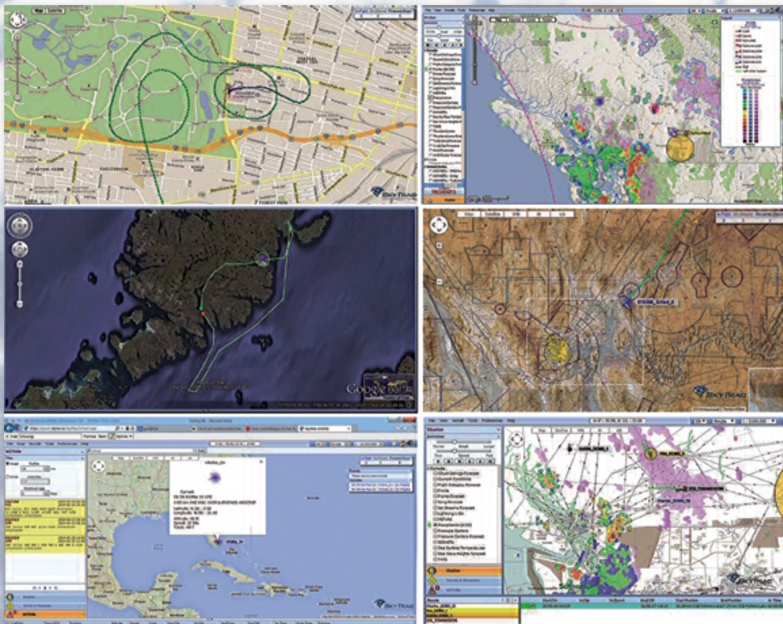
Figure 3. SkyWeb mapping options (Google maps with high resolution tracking data, satellite imagery, VFR/IFR charts. Also showing weather overlays and NOTAMS)
