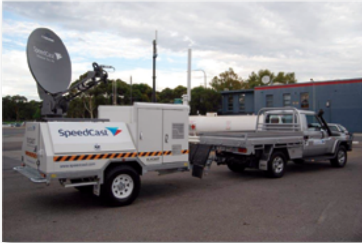
ReadyCONNECT™TA12 is a mobile VSAT solution that combines portability and rapid deployment equipment, providing instant access to the Internet, wireless and voice applications.
