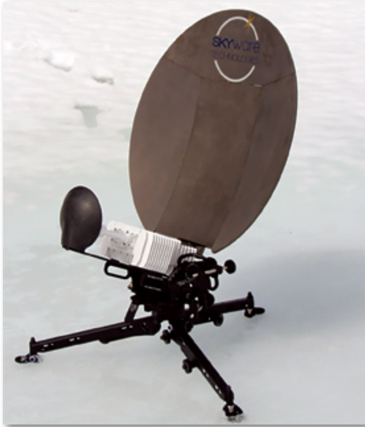
Figure 2. The Skyware Technologies ATOM 65 Ka-band Transportable Terminal
