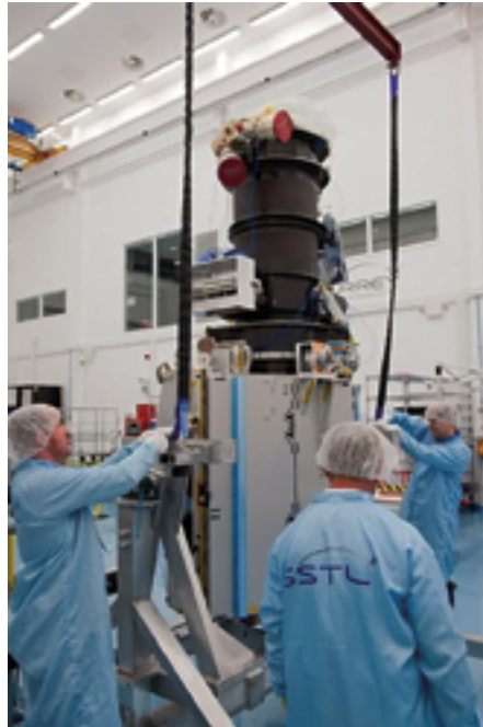
Attaching the crane hooks to the frame. Photo is courtesy of SSTL.
