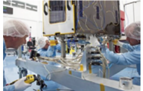
Final tiny adjustments are made to bring the spacecraft down onto the new frame in exactly the right position so that it can be safely secured. Photo is courtesy of SSTL.
