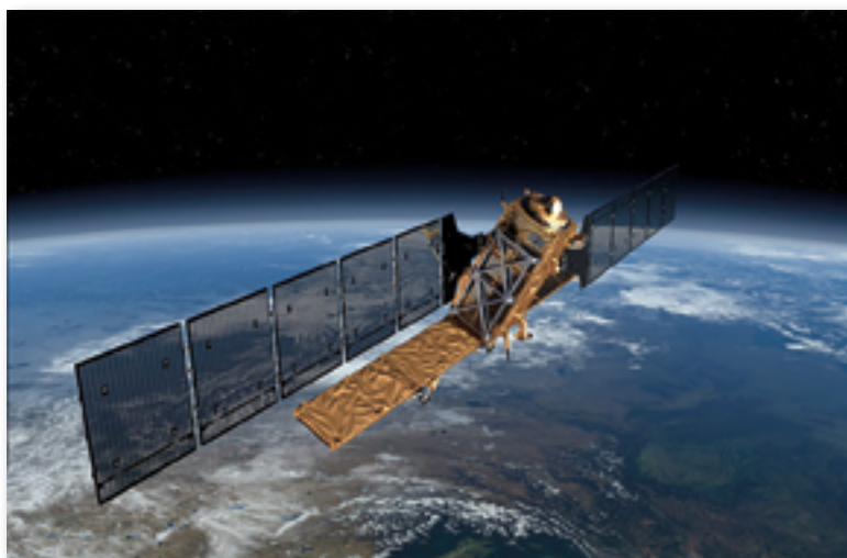
Sentinel-1, the first Earth observation satellite to be built for Europe's Global Monitoring for Environment and Security 'Copernicus' program. It is a C-band imaging radar mission to provide an all-weather day-and-night supply of imagery.
