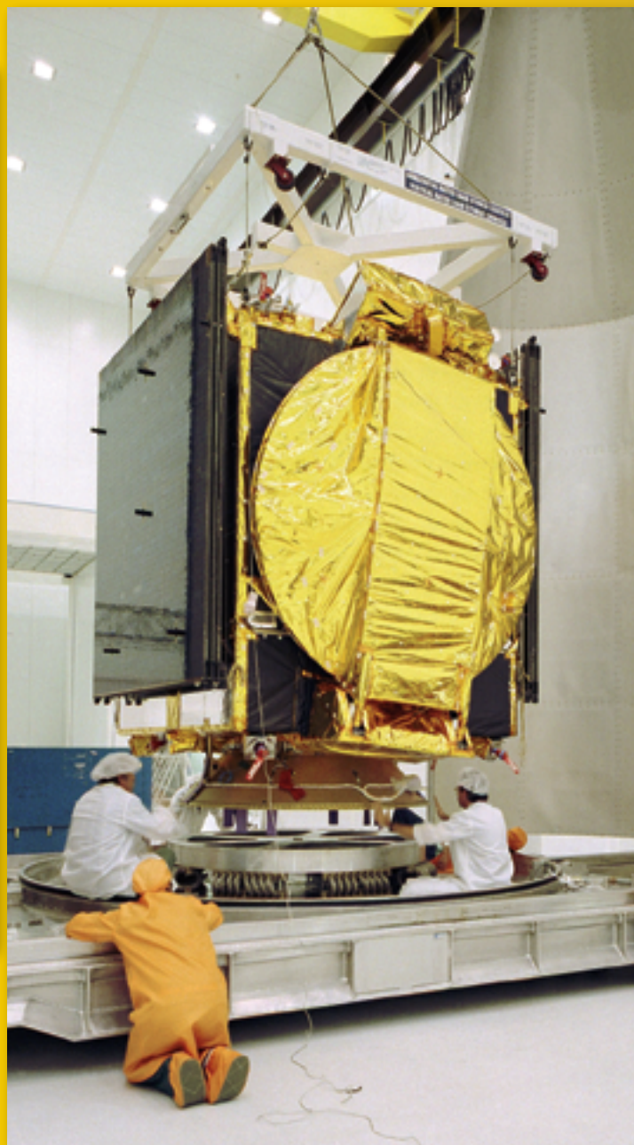
The first SSL 1300 satellite, SUPERBIRD-A, is prepared for enclosure in the Ariane 4 fairing. The satellite was successfully launched on June 5, 1989. Photo is courtesy of Arianespace.
