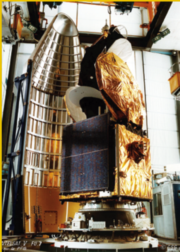
Intelsat 507 being inserted into the Ariane 1 fairing. Launched in 1983, Intelsat 507 was the first SSL mission with Arianespace. Photo by Arianespace.
