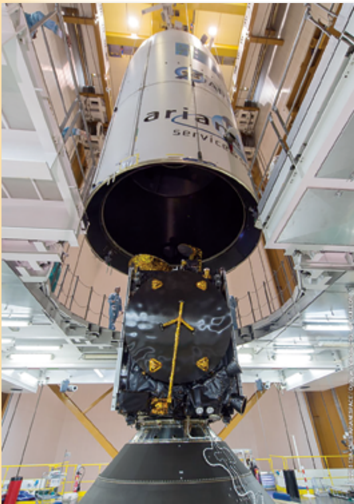
The upper payload component—containing Australia's Sky Muster spacecraft mounted on the SYLDA dispenser system, both of which are enclosed in an ogive-shaped fairing—is lowered over the ARSAT-2 satellite for Argentina, which is installed atop Ariane 5's central core.
