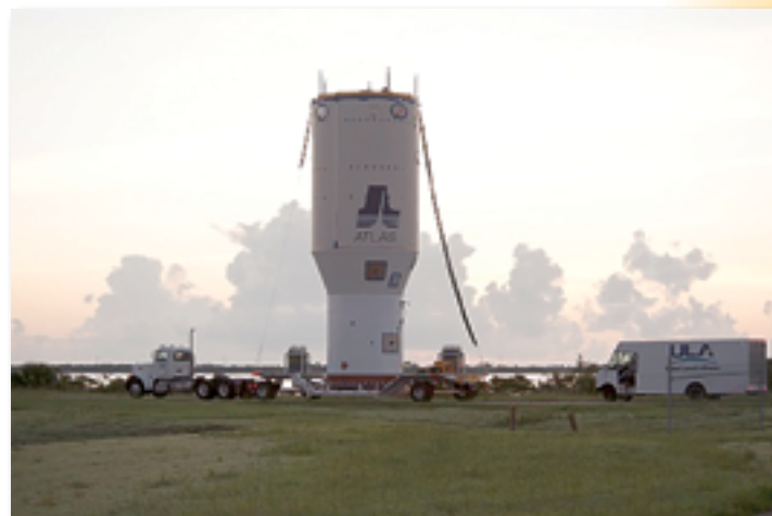
United Launch Alliance transports a five-story stack of rocket hardware approximately six miles from the Delta Operations Center to the Vertical Integration Facility using Off-site Vertical Integration.
