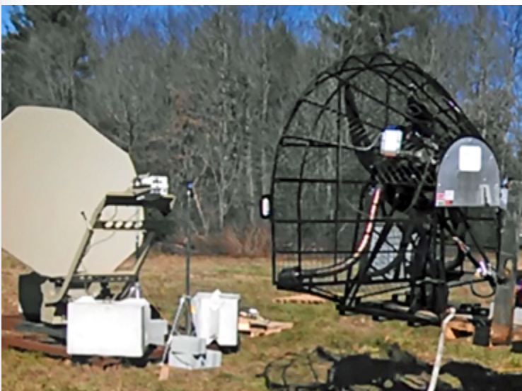
An AvL antenna getting set for a wind test using an air boat’s fan. Photo is courtesy of AvL Technologies.
