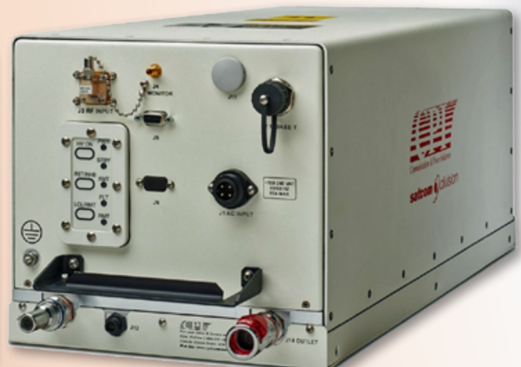
500/550 W Ka-band TWTA with liquid cooling configuration. Liquid intake and discharge connectors are on the bottom. As fans are not required in this configuration, the amplifier is smaller than air-cooled amplifiers.
