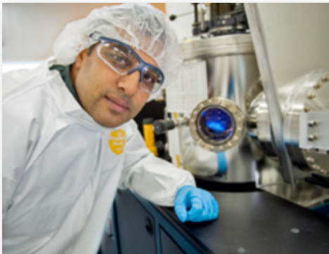
Technologist Vivek Dwivedi, who is standing in front of a sputtering reactor used to deposit vanadium-oxide onto sample substrates for testing, is collaborating with Brigham Young University researchers to develop a radiator ideal for small spacecraft. Photo is courtesy of NASA/W. Hrybyk.
