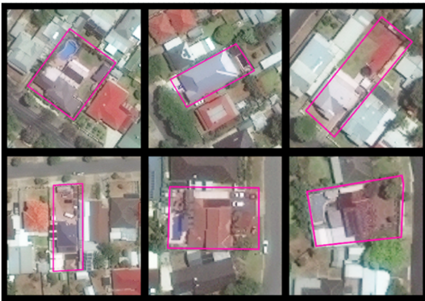
Each of the above images contains a pool inside the pink polygon. Note the variability of color, location, size, and visibility. PoolNet is a classifier implemented on GBDX that relies on a convolutional neural network and vast amounts of crowdsourced training data to distinguish properties that contain swimming pools. [Photo: DigitalGlobe]
