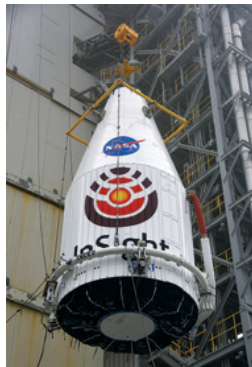
A crane hoists NASA's InSight lander inside its fairing for mating atop a ULA Atlas V rocket. Photo is courtesy of the USAF's 30th Space Wing.
