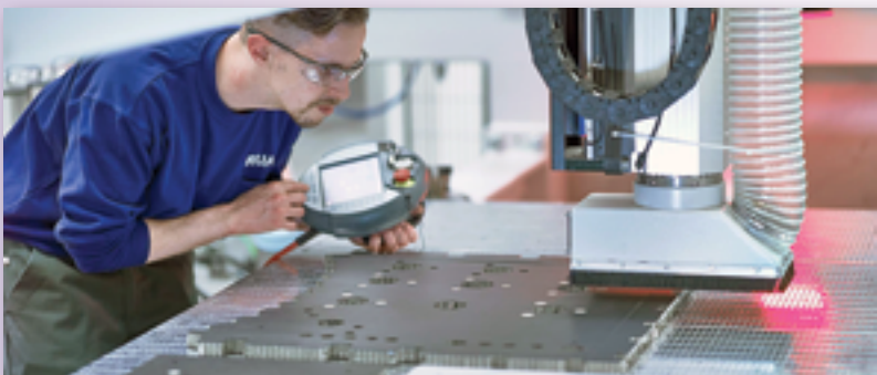
RUAG's Automated Potting Machine (APM).
