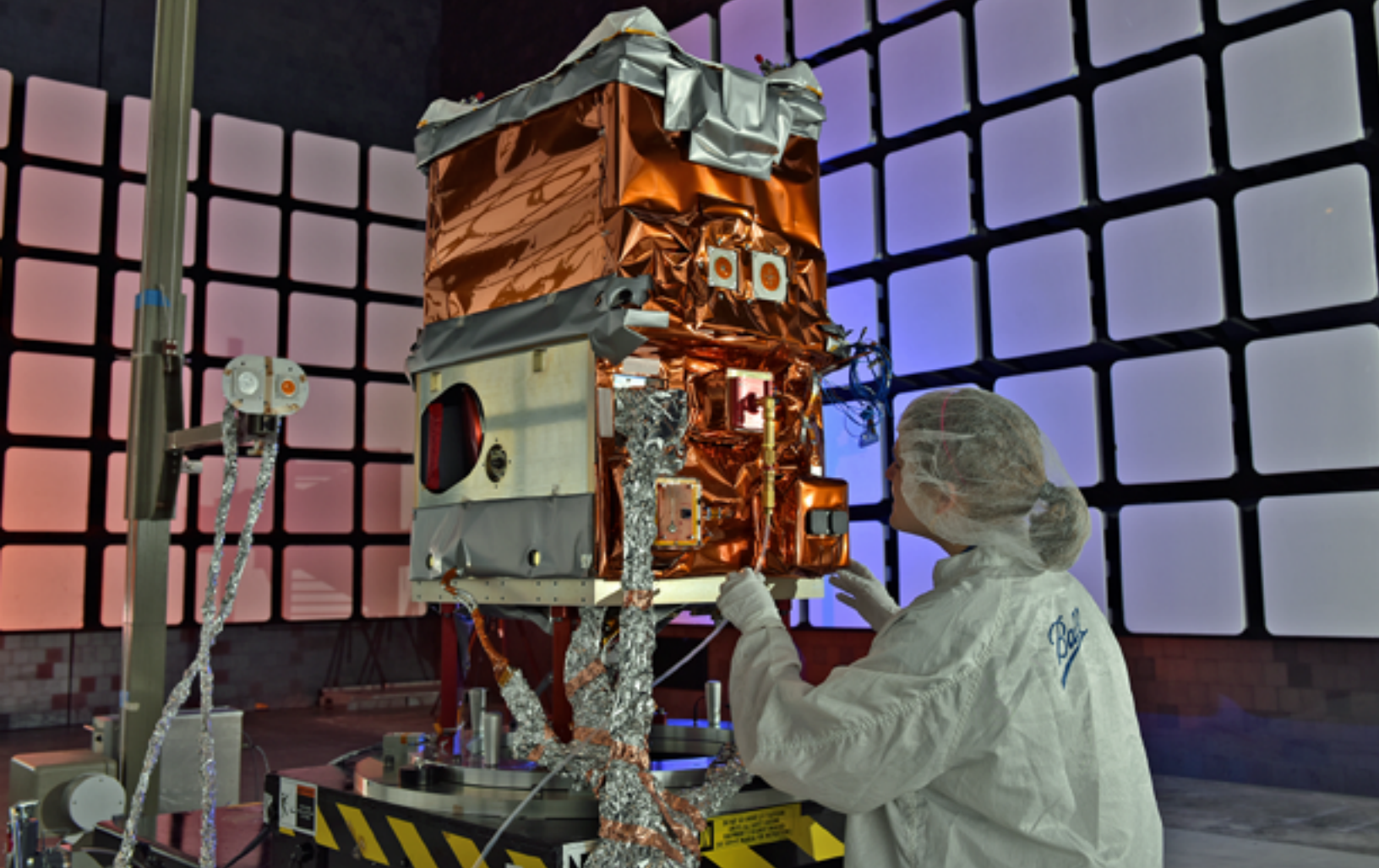
A Ball technician prepares the GPIM spacecraft in the Electromagnetic Interference (EMI) testing chamber. GPIM will validate a new high-performance spacecraft propellant, a safer and more fuel-efficient alternative to hydrazine. Photo is courtesy of Ball Aerospace
