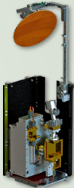
OMS MiniRad cubesat radiometer. Cost: $100k, 10x10x15 cm, 2 kg., 5 W power.
