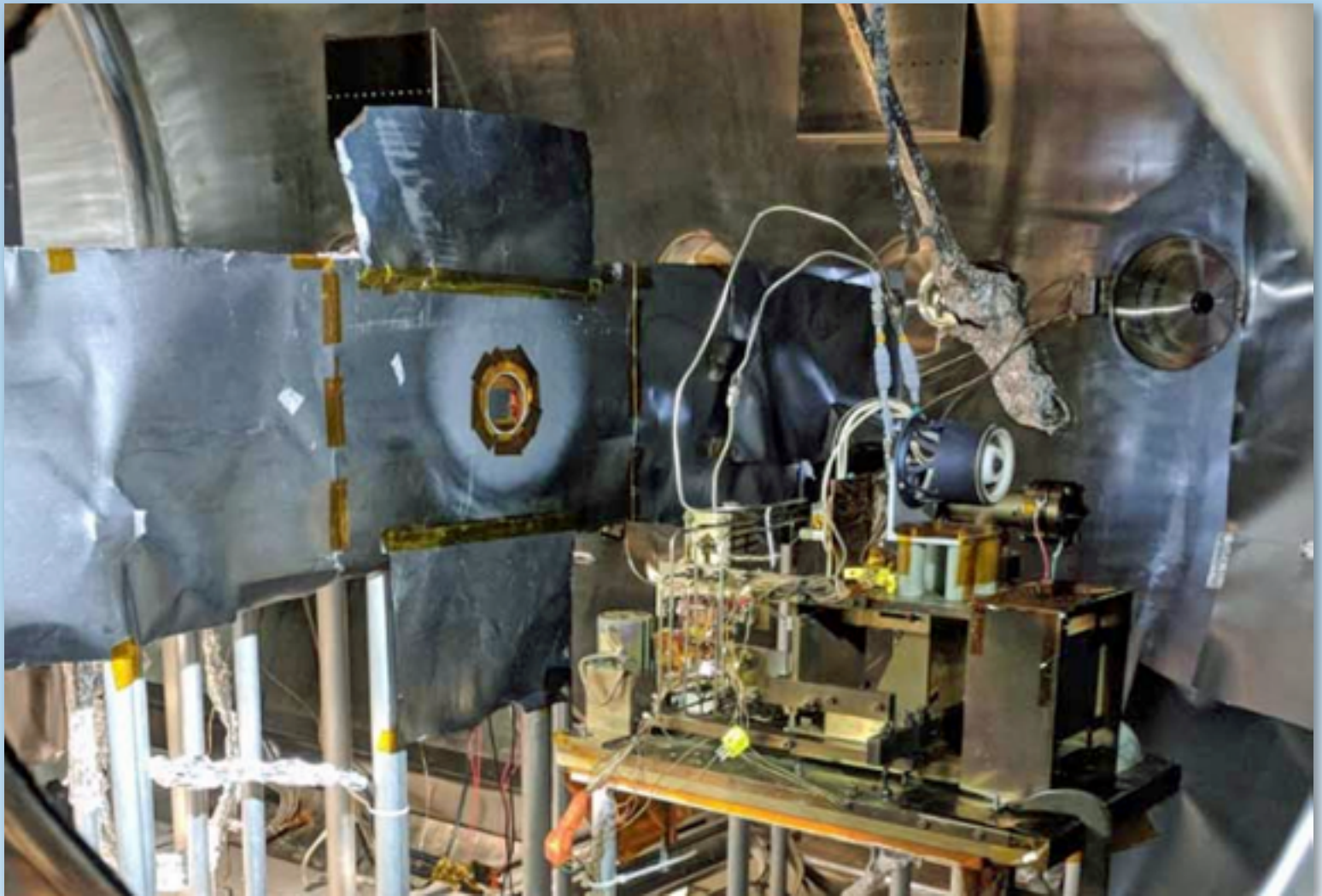
Apollo recently tested their ACE thruster in an independent lab at The Aerospace Corporation where thrust, Isp, and efficiency measurements closely matched Apollo’s own lab tests. These results confirmed that ACE has 3x better impulse per kg and 3x better impulse per liter than competing thrusters.
