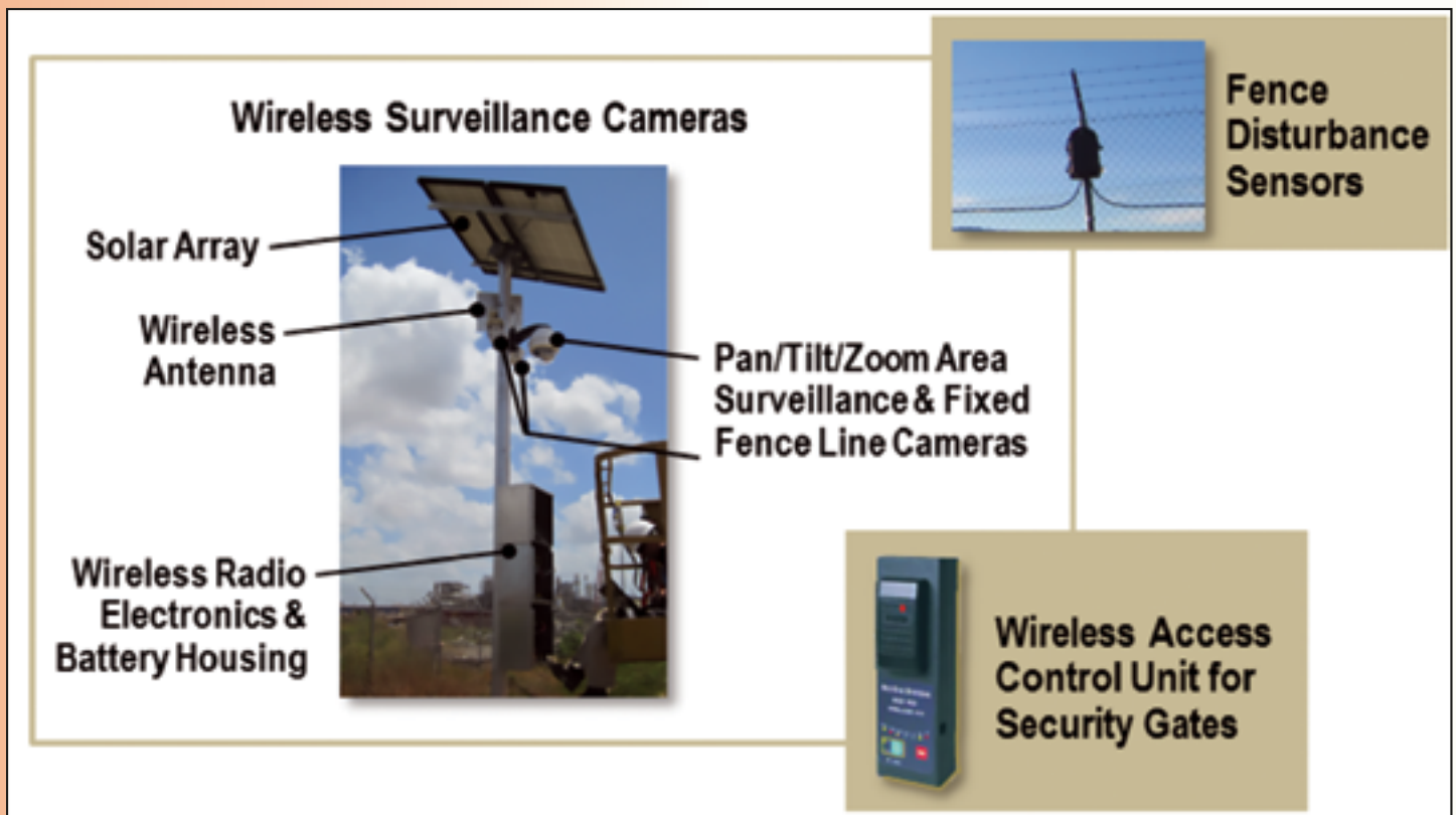
Figure 4. Typical Site Perimeter and Access Control Outdoor Elements Suitable for Wireless Connectivity to a Central Security Station
