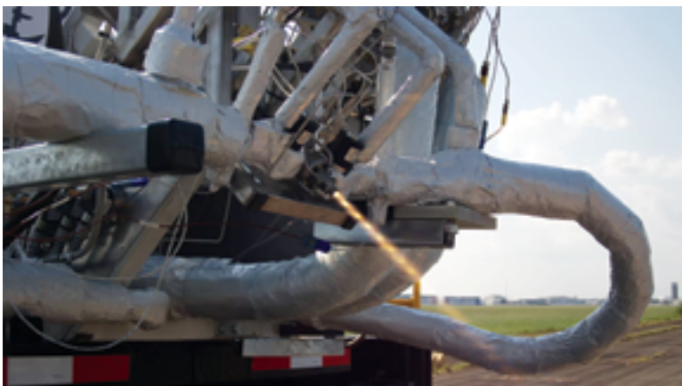
A test firing of the main lander engine. Image is courtesy of Intuitive Machines.
