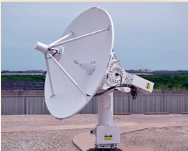
CPI ASD's three-axis 5 meter S- and X-band antenna system with a Cassegrain X-band feed and prime focus S-band feed.
