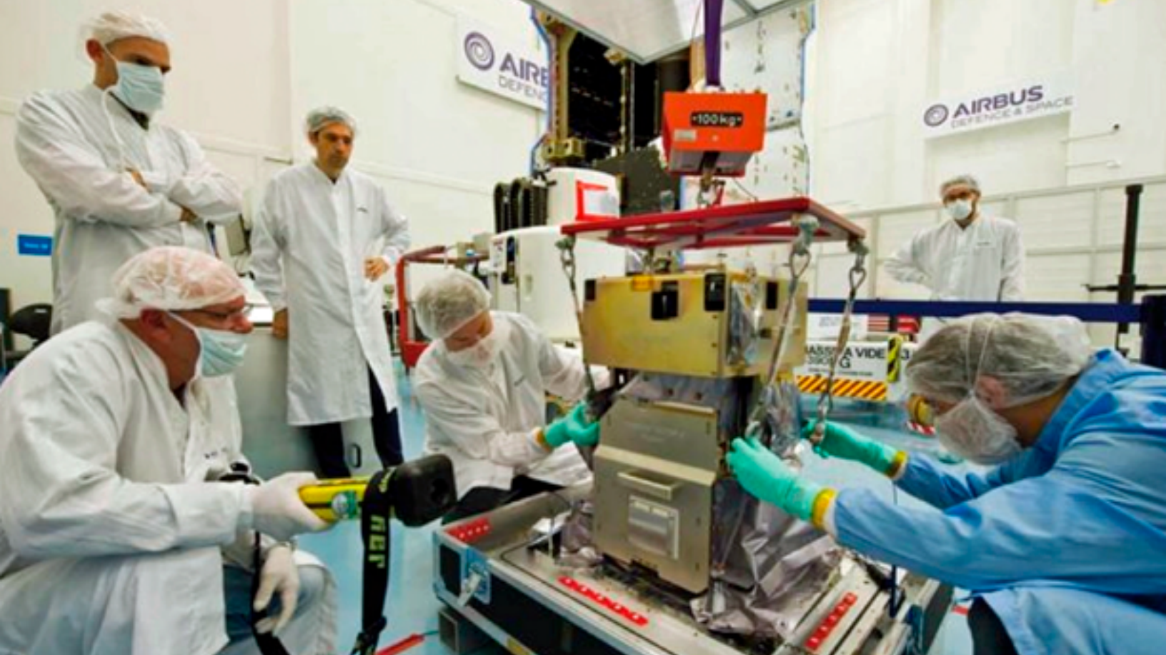
The GOLD payload is an ultraviolet (UV) imaging spectrograph designed to measure densities and temperatures in Earth's thermosphere and ionosphere. Photo of work on GOLD is courtesy of Airbus Defence and Space.
