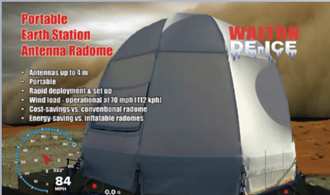
Figure 5. This image shows an example of field tests of a Portable Radome product for 1.8m antennas during wind survival testing. The photo shows a 2.4 x 2.9m (10' x 8') class Walton satellite antenna Radome that was tested with 85 mph wind loads.
